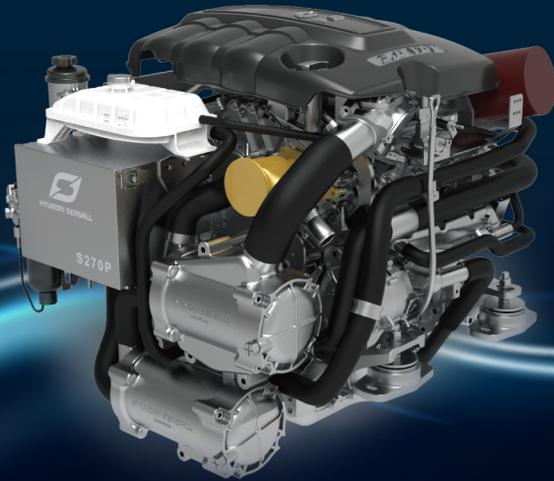
Our Piezo controlled common rail injection system delivers 270PS and 57.6kg-m torque from the 3.0 liter V6 CRDi engine. The advanced design also makes it ultralight, quiet and fuel-efficient with extremely compact dimensions.
